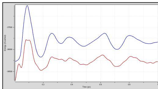
Fig.1. Plot of total energy(blue curve) and potential energy( red curve) against time
