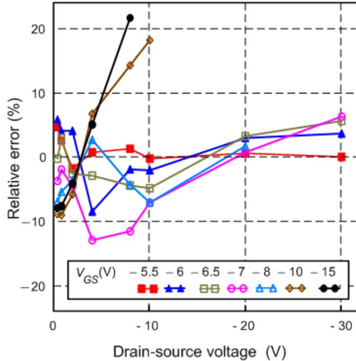
Fig. 1. Relative error as a function of applied voltages for  $p$ -channel MOSFET FQD5P20. All graphs of the function  $\delta(V_{DS})$  intersect with the zero level, what indicates a good quality of the model (4) – (5).
