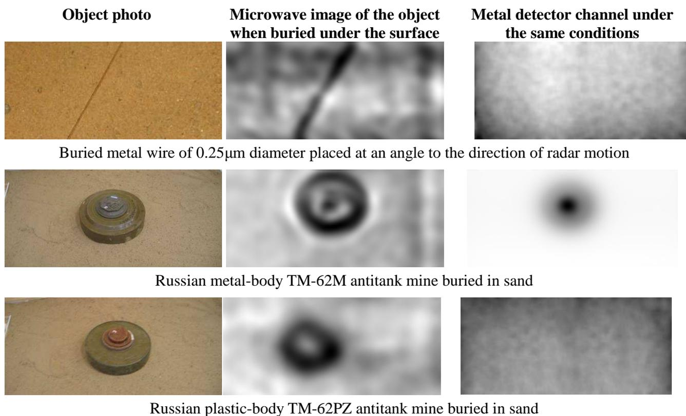
Fig. 28. Images recorded by subsurface radar and metal detector.
