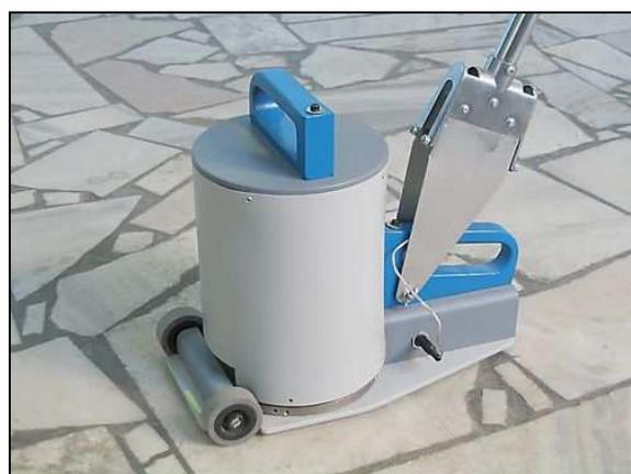
Fig. 13. RASCAN-4/2000 radar head.
