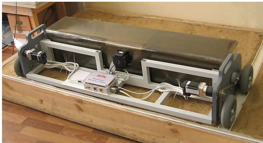
Fig. 27. Holographic radar with electro-mechanical scanner. ISTC project #2541.
