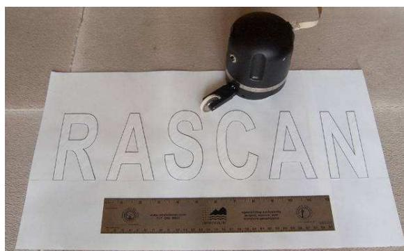
Fig. 7. Paper sheet with embedded letters that form the word RASCAN. Metal ruler is 12 inches (30.48 cm).
