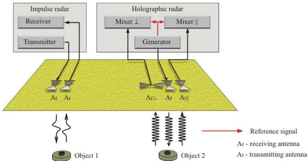
Fig. 3. Comparison of impulse and holographic radars schemes
