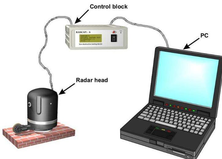
Fig 4. Connection scheme of the RASCAN-4 radar parts with computer.
