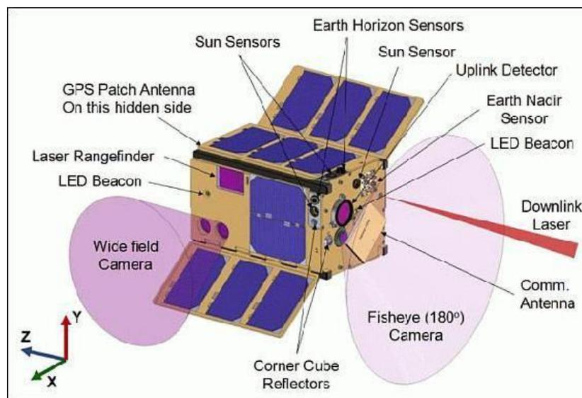
Fig.1: Schematic rendering of AeroCube-OCSD nanosatellite (image credit: The Aerospace Corporation) [9].
