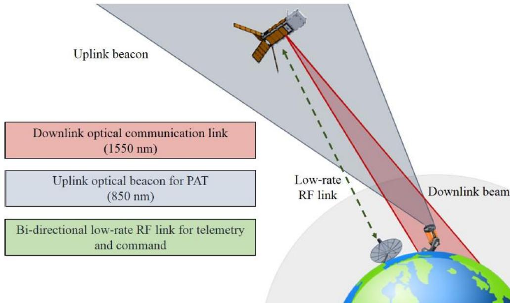
Fig.5: NODE system architecture, consisting of a 1550-nm downlink beam as primary downlink method, a 850-nm uplink beacon for acquisition and tracking, and a bi-directional radio-frequency link for telemetry and command [25].
