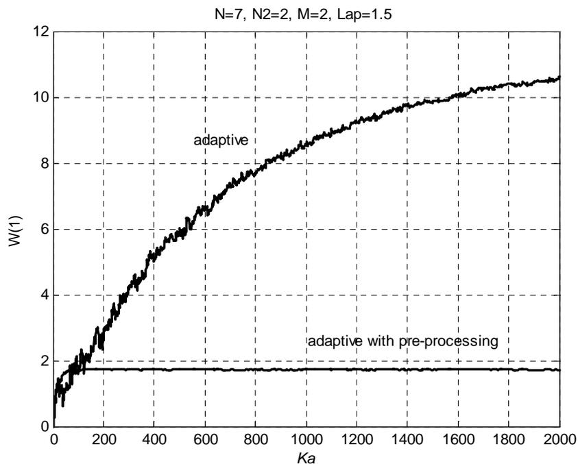
Figure 5. Adjustment of weight at adaptation with preprocessing
