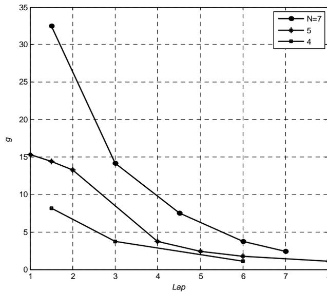
Figure 7. Dependence of minimum eigenvalues ratio on aperture size
