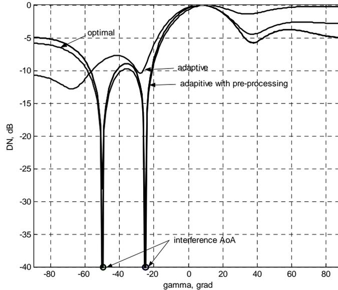
Figure 6. Antenna pattern nulling and adaptation with preprocessing
