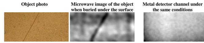
Buried metal wire of  $0.25 \mu m$  diameter placed at an angle to the direction of radar motion
