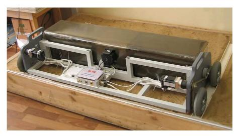
Fig. 27. Holographic radar with electro-mechanical scanner. ISTC project #2541.
