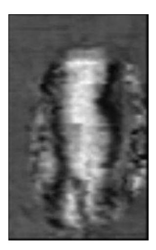
Fig. 19. Radar image of the medallion at the frequency of 3.9 GHz.
