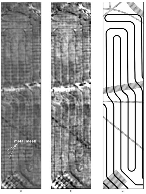
Fig. 16. Interpretation of the radar image: a) raw radar image at the frequency of2.0GHz (cross polarization); b) image "a" after Fourier-based numerical filtration;c) layout of pipes and communications on results of the radar's surveying
