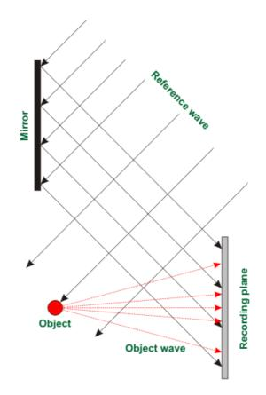
Fig. 2. Diagram of optical hologram with an inclined light beam.
