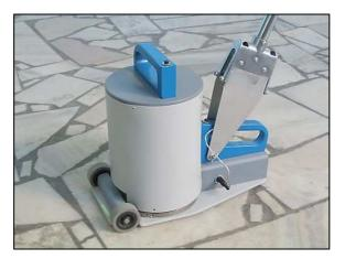
Fig. 13. RASCAN-4/2000 radar head.
