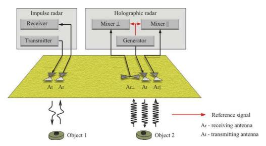
Fig. 3. Comparison of impulse and holographic radars schemes
